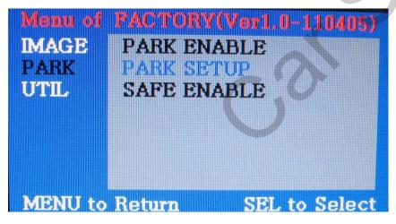
② If you press "UP" button on the keypad about 2 seconds long, you can see the left image on the screen. Now that you choose "PARK SETUP" and press "OK" on the keypad, you can control the width of the rear parking guide line.
