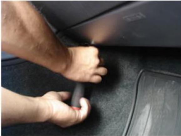
① Remove screws on Glove box.
